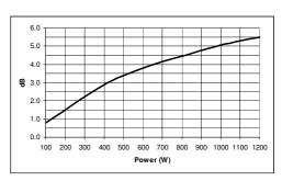
Note: These losses are calculated from a five minutes AES power test applying band limited pink noise (50-500 Hz). The loudspeaker is free-air standing.
