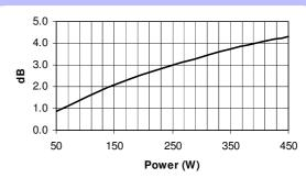
Note: These losses are calculated from a five minutes AES power test applying band limited pink noise (120-3500 Hz). The loudspeaker is free-air standing.
