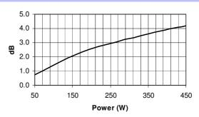
Note: These losses are calculated from a five minutes ALS power test applying band limited pink noise (120-3500 Hz). The loudspeaker is free-air standing.
