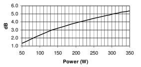
Note: These losses are calculated from a five minutes AES power test applying band limited pink noise (25-1200 Hz). The loudspeaker is free-air standing.
