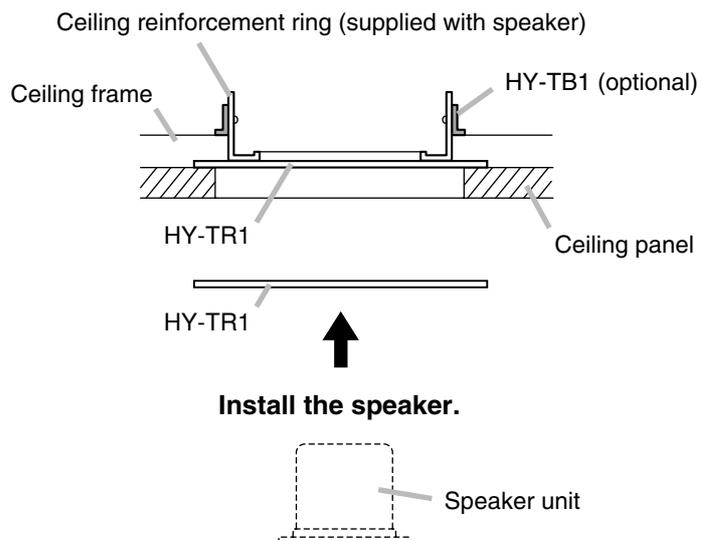
If the Trim Ring cannot be installed on the back side of the ceiling, cut the ring as shown in the illustration below.
