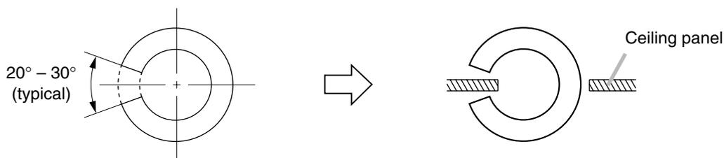
**Note:** The cut-out section facilitates insertion of the Trim Ring through the mounting hole.
